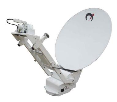
The Sat-Lite Technologies Model 1256 vehicle-mount antenna is a high performance design for VSAT or SNG applications in a compact design. Key features include a low stow height configuration and compact pedestal minimizing vehicle constraints. Also included is an integrated auto-locate controller with manual override. The integrated control system includes an option for a programmable digital video receiver that can be used to positively identify the satellite and automatically peak the antenna.
